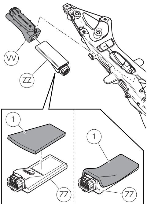
Apply the heat insulator (1) on the Black Box ECU (ZZ), centring heat insulator centreline with ECU centreline, and press it firmly to make it adhere on the whole surface. Insert the thus heat-insulated Black Box ECU (ZZ) onto the Black Box mount (VV). Connect the Black Box power connector, and refit the Black Box ECU assembly (ZZ) inside subframe.
